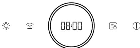
There are five buttons on the front panel as shown above: Illumination, Hood-Hob Linkage, Wake-Up (also touch this button to adjust the airflow), Lock-Screen, Delay/Stop. For the first time to start the hood, please press the Wake-Up button first and then touch the ring clockwise and the airflow will get bigger and bigger. When the whole ring is red, it starts to suck at the highest speed.
